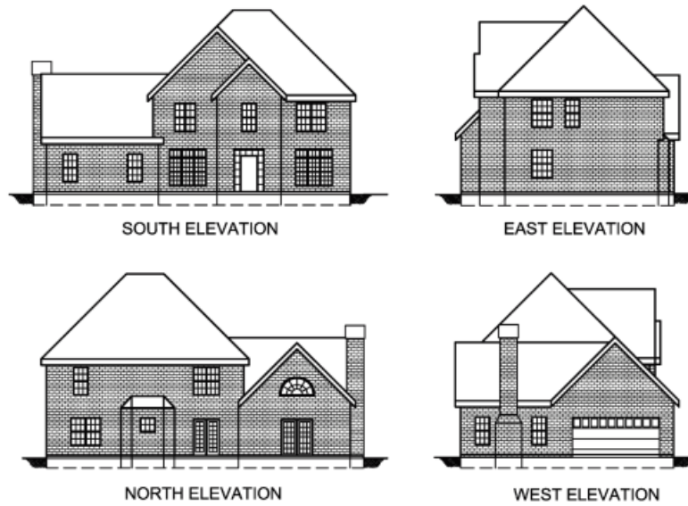
Figure C-2 Model dwelling elevations showing full anchored brick veneer and slab-on-grade configuration.
