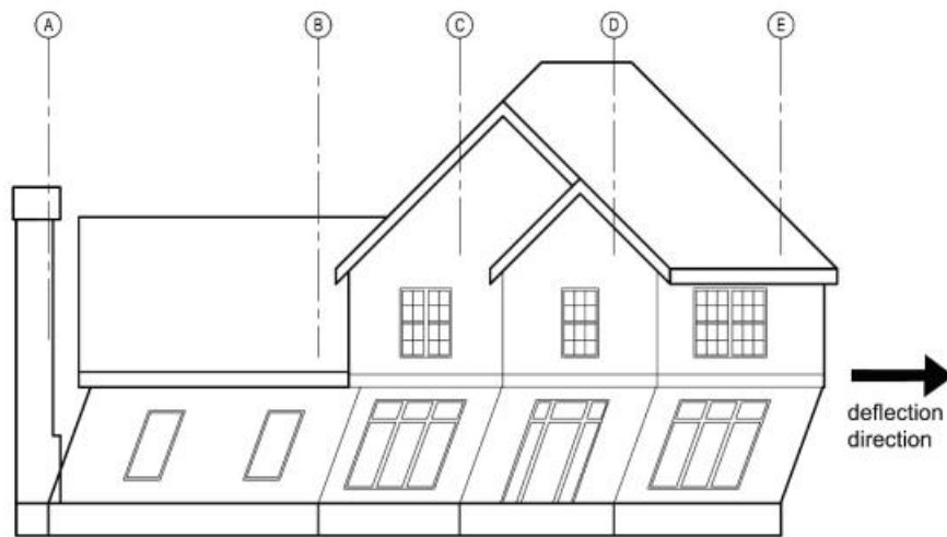
Figure 2-19 Change in deformation patterns associated with soft-story irregularity
