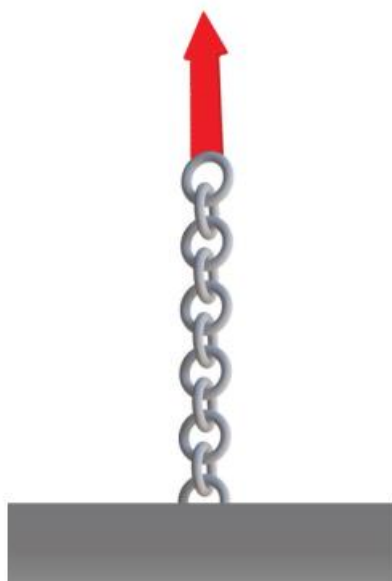
Figure 2-7 Chain illustrating the load path concept.
